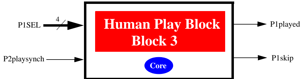
Figure 12. The detailed view of the input and output signals of the Human Play Block.
