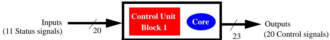
Figure 10. Inputs and outputs of the Ppm control unit.
