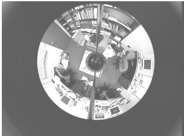
Figure 3: An image taken by the parabolic omnidirectional camera. This is the scene where the motion experiments were conducted.
