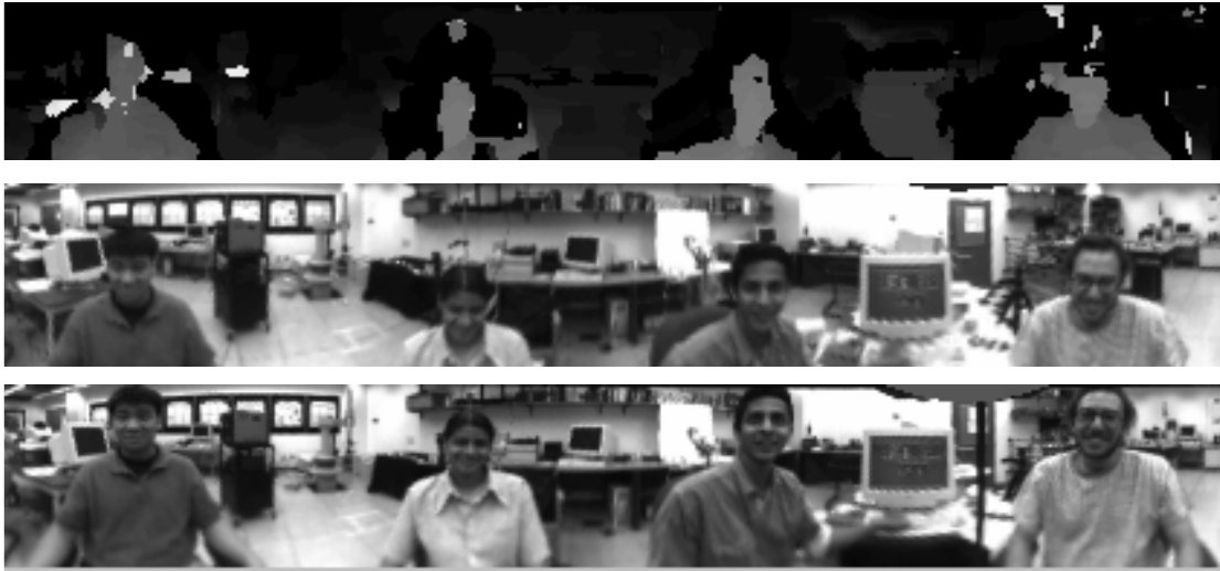
Figure 9: Panoramic images and disparity map. The disparity map (on top) was computed from the two panoramic images (on bottom).
