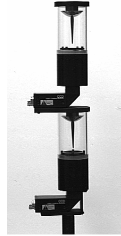
Figure 8: A compact panoramic stereo camera. In this design we used parabolae with a 360^\circ \times 200^\circ field of view.
