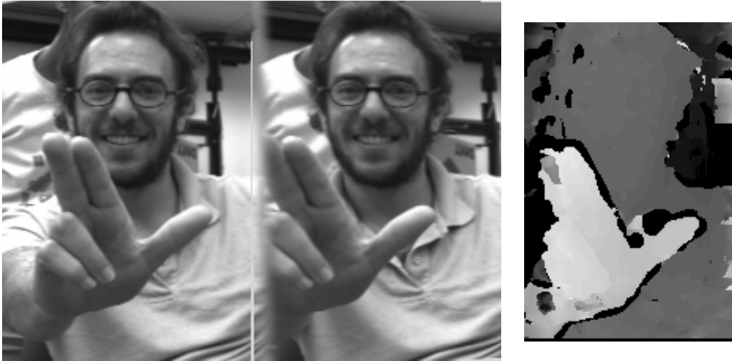
Figure 5: Stereo image and depth map. On the left is an image taken by a catadioptric stereo system and on the right is the depth map computed with a 7 \times 7 correlation window.
