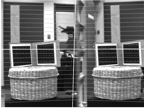
Figure 4: Estimated epipolar geometry. The epipolar geometry was computed using the 8-point linear algorithm and then enforcing the planar motion constraint by non-linear minimization. The two bright lines indicate the estimated horizon line of the planar motion and the estimated image of the screw axis (intersection of the mirrors).
