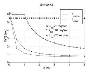
(a) The bottleneck is given by the limited bandwidth on the access link of the national cache.  $\beta_N S = 0.9 \cdot C_N$
