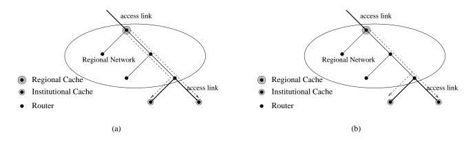
Figure 12: Caching distribution (left) and Multicast distribution (right).
