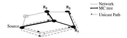
Figure 1: Network topology with multicast tree.
