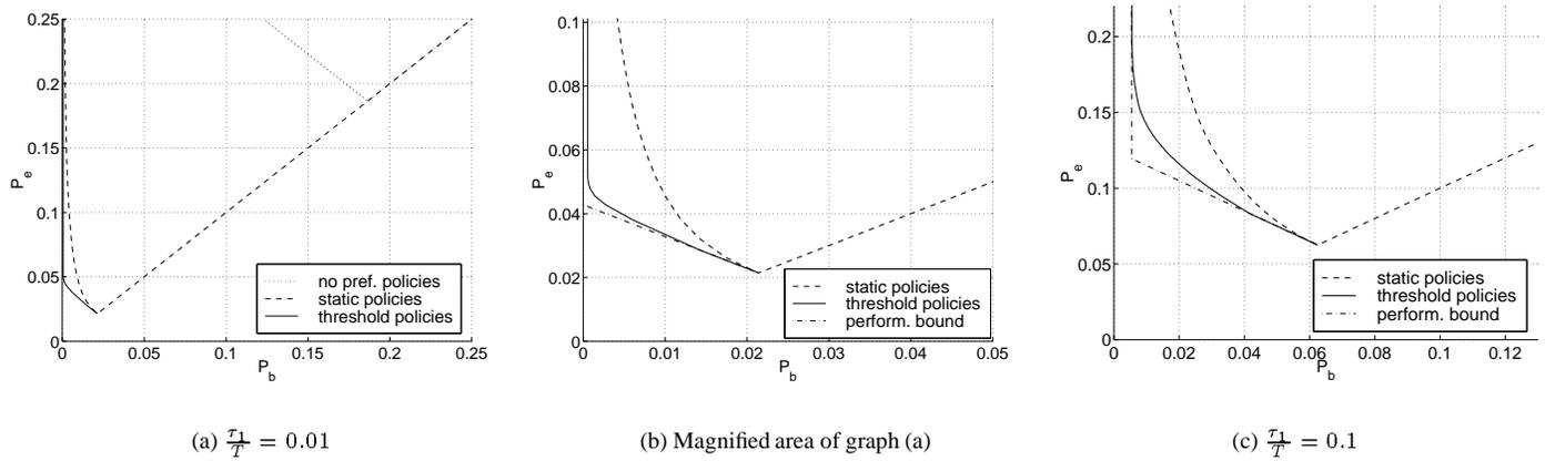
Fig. 5.  $(P_b, P_e)$  tuples for three types of streaming policies: no-prefetching policies, static policies and threshold policies.
