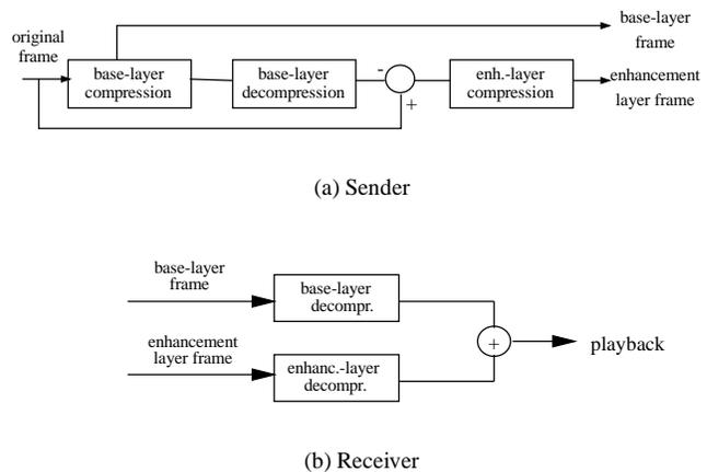
Fig. 1. Layered encoding and decoding of video.
