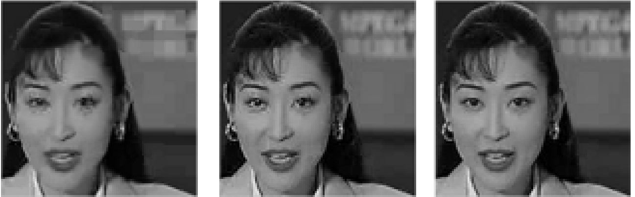
Figure 11: frame 140 of Akiyo when (left) (X_{140} = 0, X_{141} = 0) – PSNR = 33 dB, (middle) (X_{140} = 3, X_{141} = 0) – PSNR = 36.3 dB, (right) (X_{141} = 3) – PSNR = 38.3 dB.
