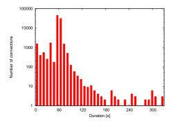
Fig. 4. Histogram of TCP connection durations
