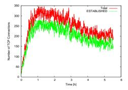
Fig. 3. Number of TCP connections present in one-second intervals
