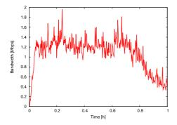
Fig. 5. Routing Table Attack: UDP Traffic at Victim Host
